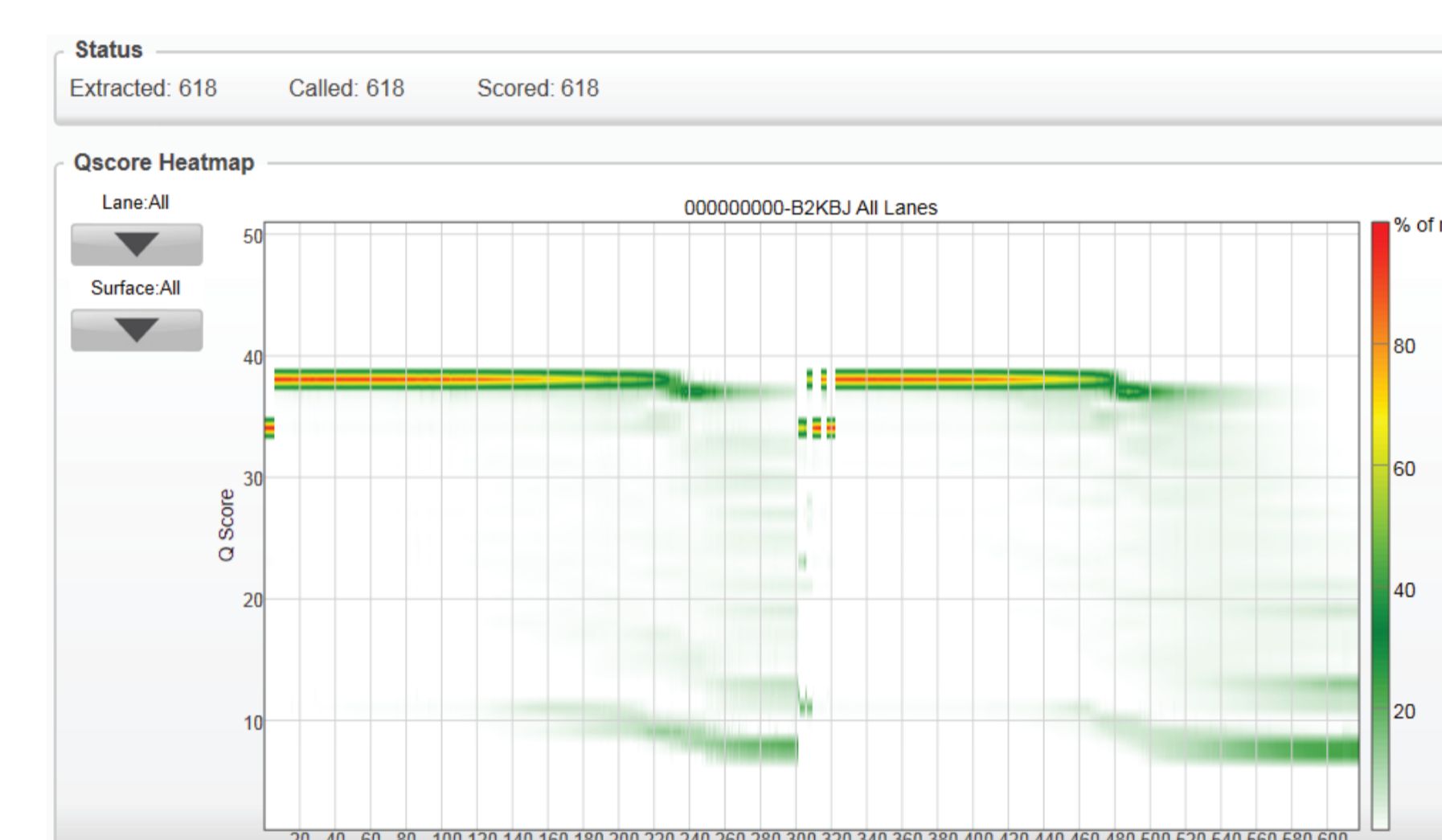
Figure 4. Quality read scores per cycle of the entire multiplexed MiSeq run, demonstrating that various reaction volumes can be run together and produce quality scores similar to conventional 2x300 genomic runs.
