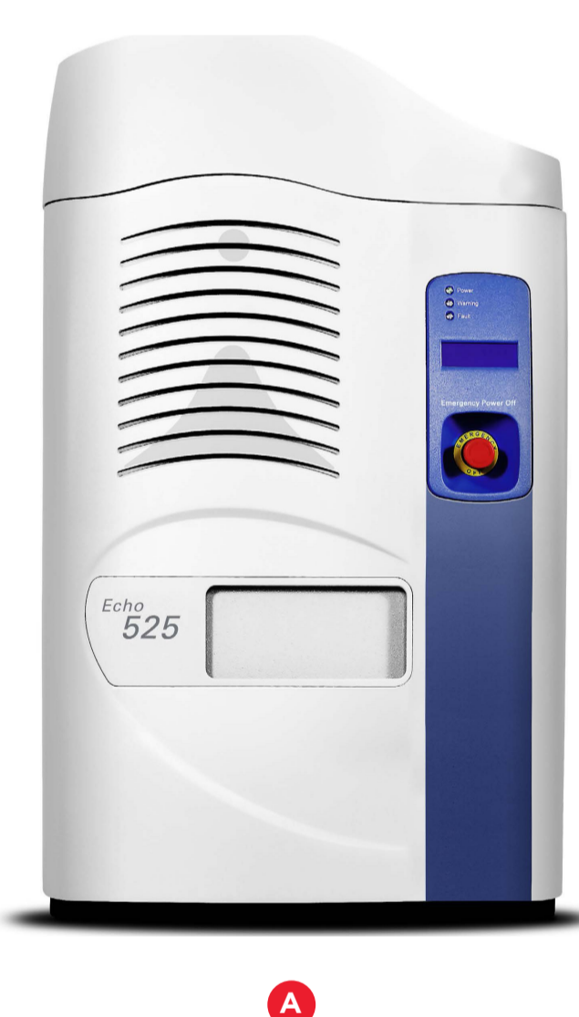
Figure 1A. The Echo 525 Liquid Handler
